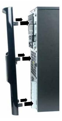
**2** Press the bezel firmly into place.
